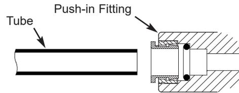
Cut tubing square with end of tubing round, smooth, with no cuts, nicks or flat spots.
