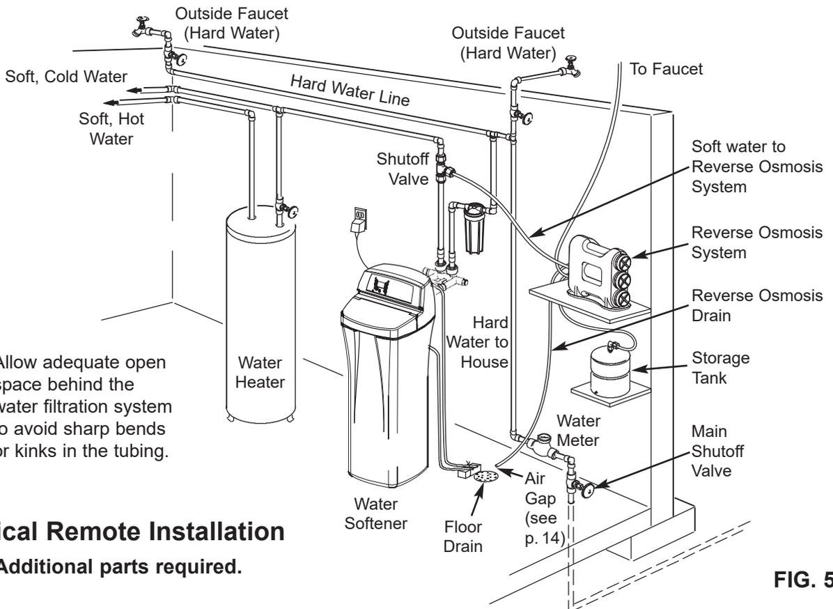
**IMPORTANT:** Allow adequate open space behind the water filtration system to avoid sharp bends or kinks in the tubing.
