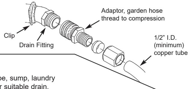
To standpipe, sump, laundry tub or other suitable drain.
