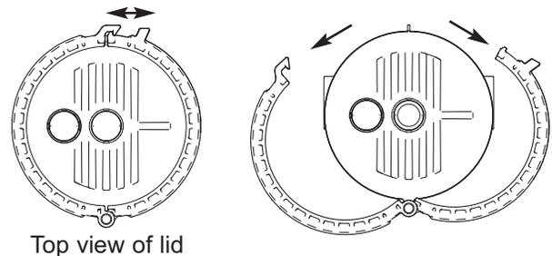
5. Swing the clamp halves open and lift the lid assembly up off the filter cartridge and sump.
