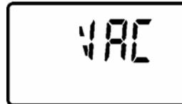
**To resume regenerations,** press (do not hold) the
