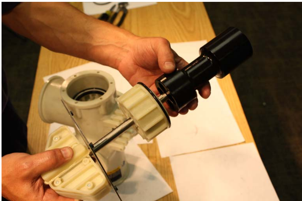
Yoke, piston, piston rod and end cap assembled
