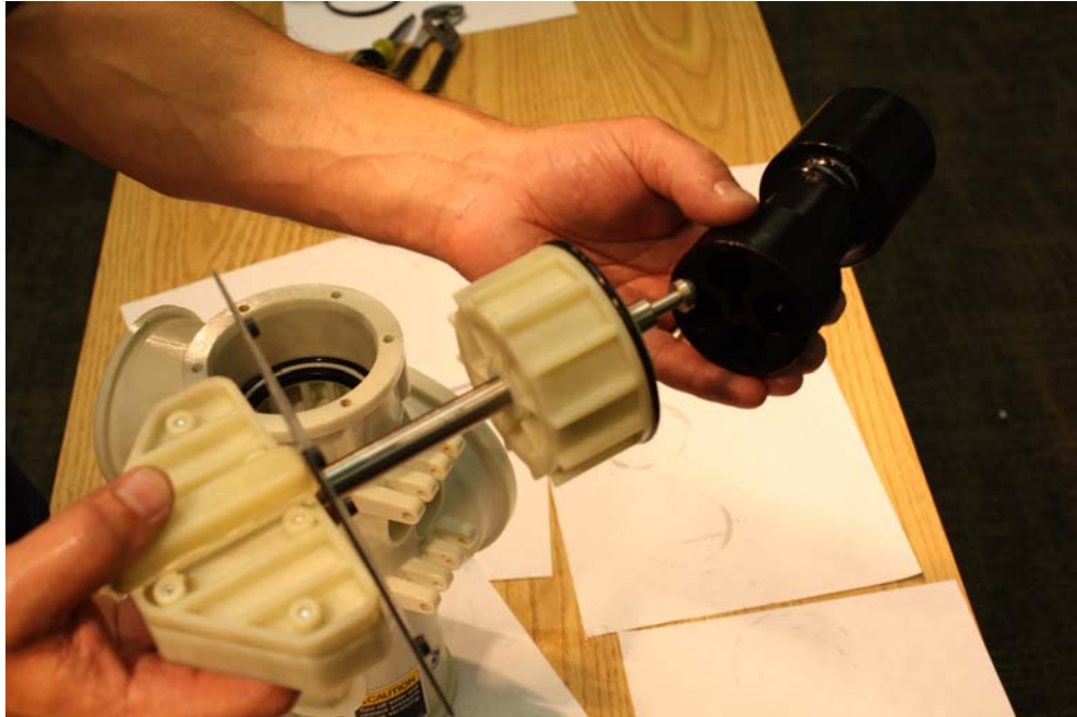
Lubricate piston and install on piston rod
