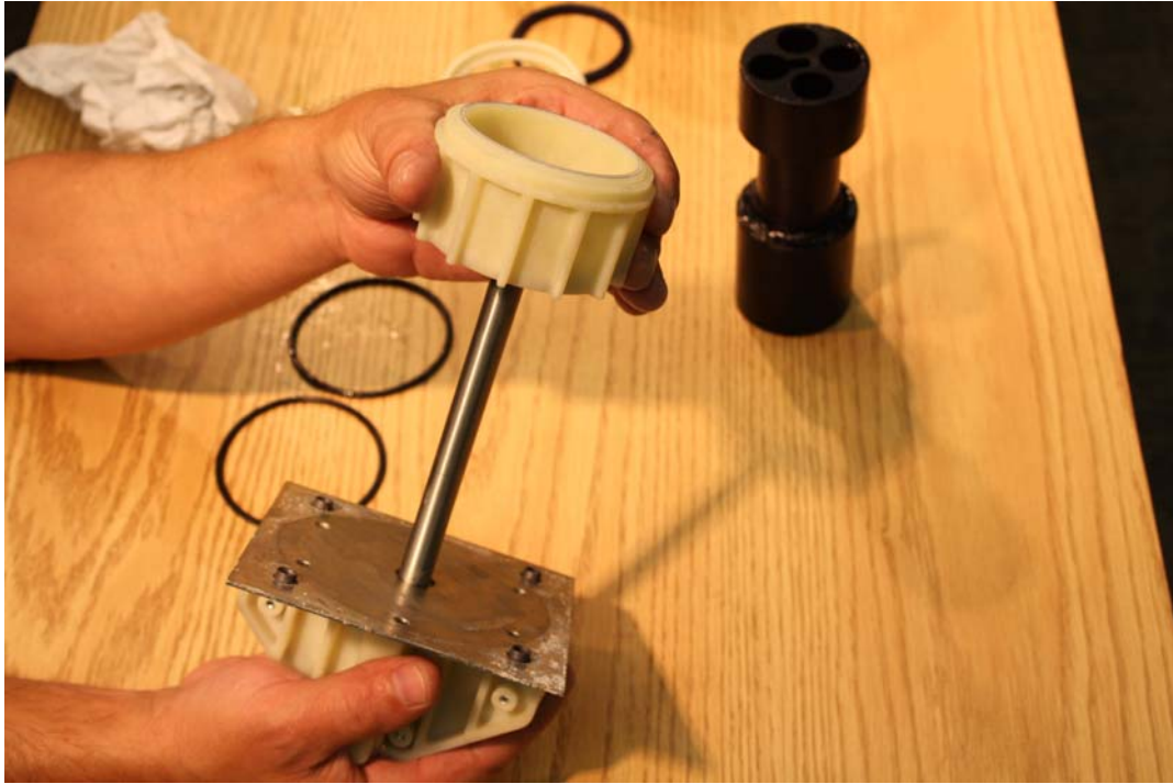
Remove end plug from shaft
