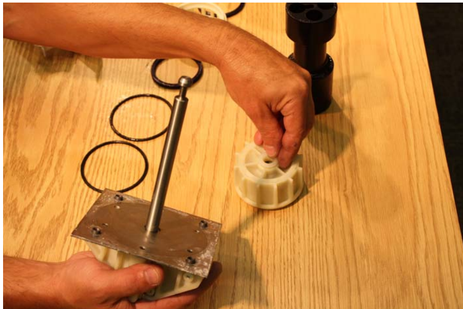
Remove end plug from shaft
